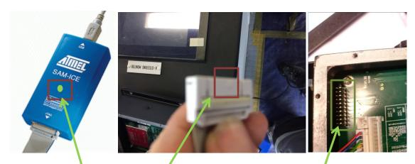
Cut the 'notch' of one end of the cable plug so that the cable can be plugged onto the Back of the CD401XX with the notch side into the metal housing. If connected correctly and power is on you should see green light on the SAM-ICE module
