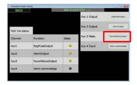
Check that Aux 3 Relay is set to 'PowerFailureOutput'
