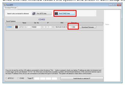
Repeat the programming with the current software (SW-M003-1.57) restart the system and check in Com setup that the software is upgraded.
