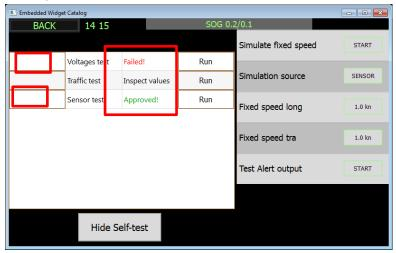
Press self test and check you have approved. On the first and last point. If you have failed press the S logo on the left and check what is wrong
