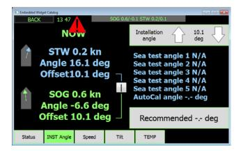
Press back and go to the INST angle reenter the Installation angle (Note if the system is in STW+SOG mode there will be 2 angles here. Press on the STW or SOG values on the left to select the set of values
