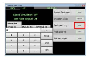
Set the Fixed speed long to 10kn (if you have no sensor installed change simulation source to JB70)
