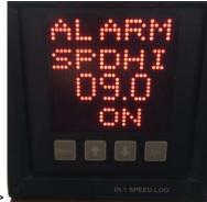
Turn on the Speed hi alarm set to 9kn
