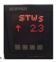
The speed will slowly raise up and down, and an alarm should be generated as the speed rises past 9kn.
